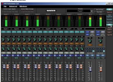
One of the dangers of using a conventional mixer in a sound system operated by an untrained sound technician is the occurrence of feedback. The more open channels there are, the greater the overall system gain and the lower the potential acoustic gain (gain before feedback).
